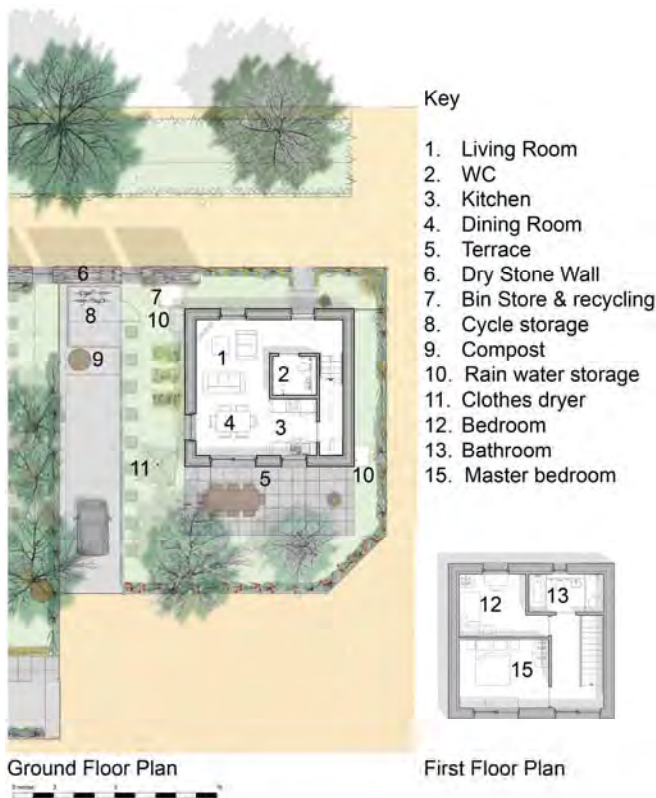
Figure 2-9. Lime house floor plans
