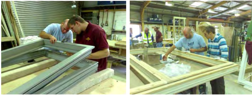
Figure 2-8. The Lime House windows being built at Custom Precision Joinery
