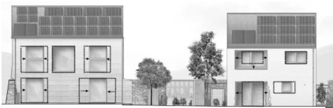
Figure 2-10. Larch and Lime House glazing ratio changes when using Manchester average weather data.
